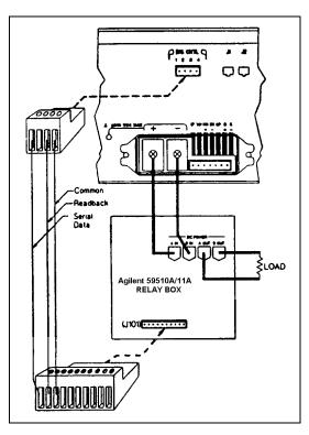
Figure D-6. Relay Link Connections
